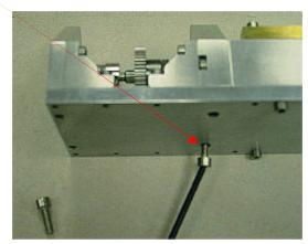
Carefully maneuver the T-Axis into the crankcase assembly.
