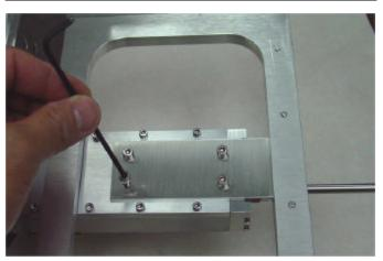
Center main shaft spur gear to motor gears and use thin 13mm wrench to tighten shaftloc.
