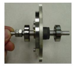
Fit test the spur gear assemblies into the crankcase with a light preload on the bearings.
