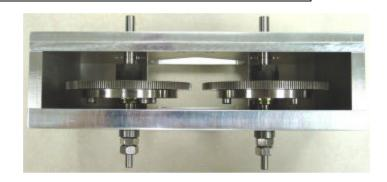
Mount crank case into inner body assembly with 'T' Flexure piece.
