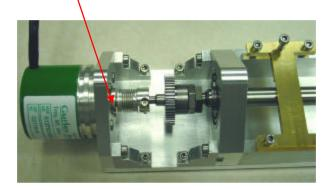
Assemble crankcase and motor spur gear subassemblies.
