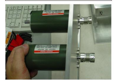
Connect motors to gear assembly with 8mm bellows couplings.
