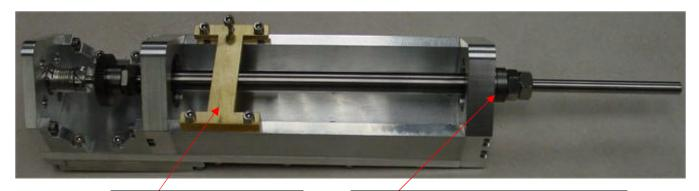
Do not tighten down brass brake piece at this time.
