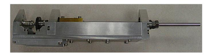
Tighten shaftloc sleeve to spur gear using thin profile wrenches.
