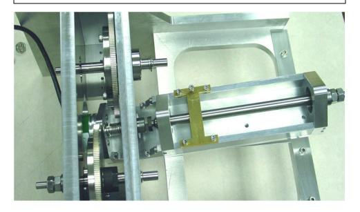
Attach T-Axis to T-Flexure plate.
