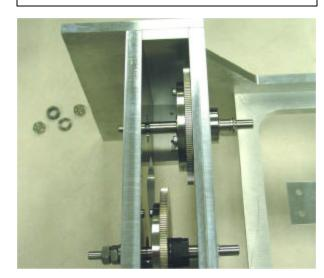
Temporarily remove the braces and mounting screws to allow for assembly into the crankcase assembly.
