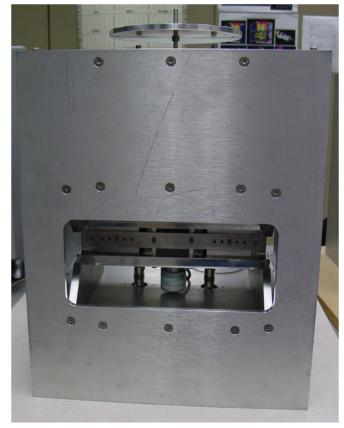
Attach load plate to main shaft with a shaftloc coupling to complete assembly.
