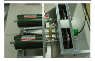
Attach the bottom case shelf and connect two Heidenhain encoders to the motor spur gear assembly
