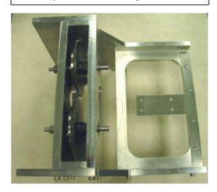
Remove the preload nuts on one of the gear assemblies and carefully slide forward.
