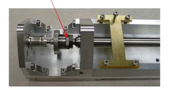
Attach 4mm bellows coupling to Gurley encoder first before connecting to shaft.
