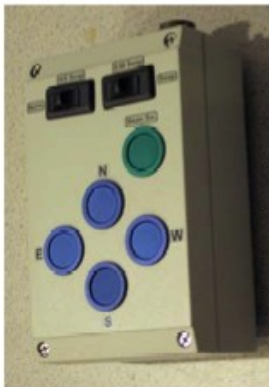
The Observer Hand Paddle. There are 2 units located in the primary observer's area and the guest observer's area.
