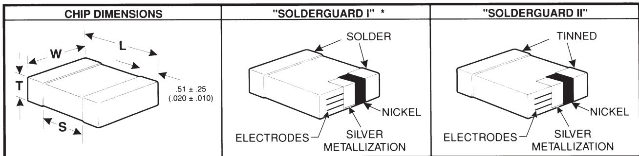
\* Add .38mm (.015") to the positive width and thickness tolerance dimensions and .64mm (.025") to the positive length tolerance dimension for Solderguard I.
