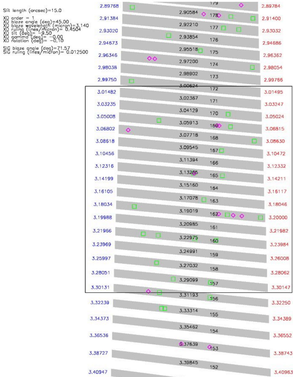
Figure 6. Exposure L2 (see Table 5), slit length 15", 450 line per mm grating. The box indicates the H2RG array.
