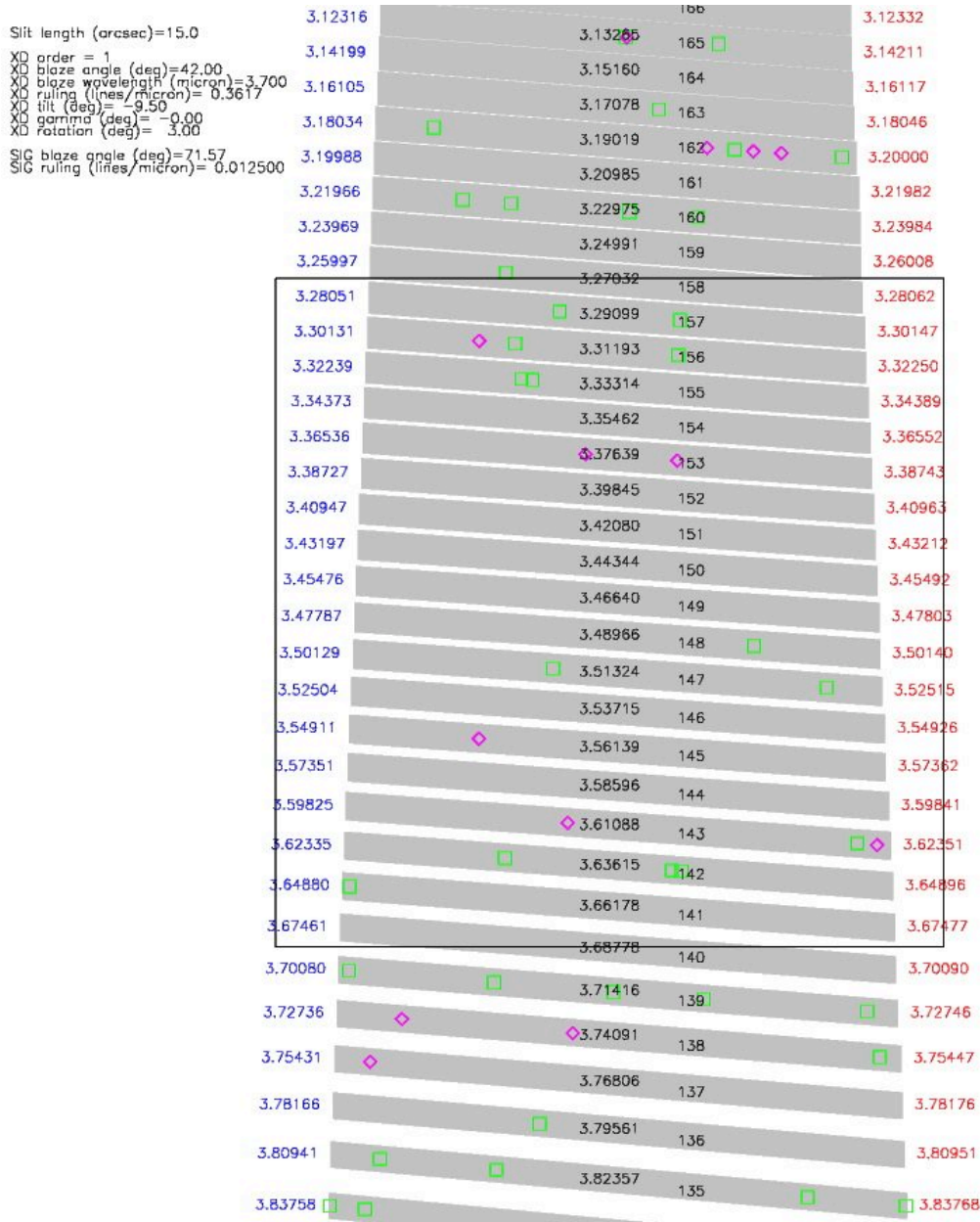
Figure 8. Exposure L4 (see Table 5), slit length 15", 360 line per mm grating. The short wavelength limit (about 3.28 \mu\text{m} ) is set by the need to keep orders separated by at least 10 pixels. The box indicates the H2RG array.
