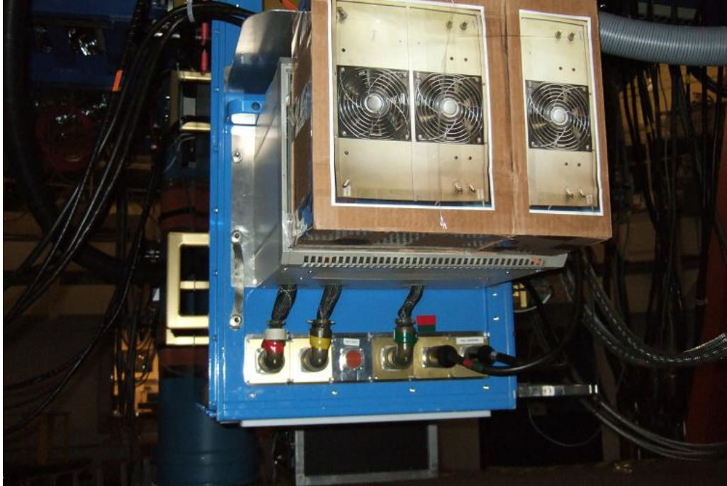
Current controller SpeX with a space model of the ARC controllers shown for comparison on (12 slot for H2RG and 6 slot for Aladdin).
