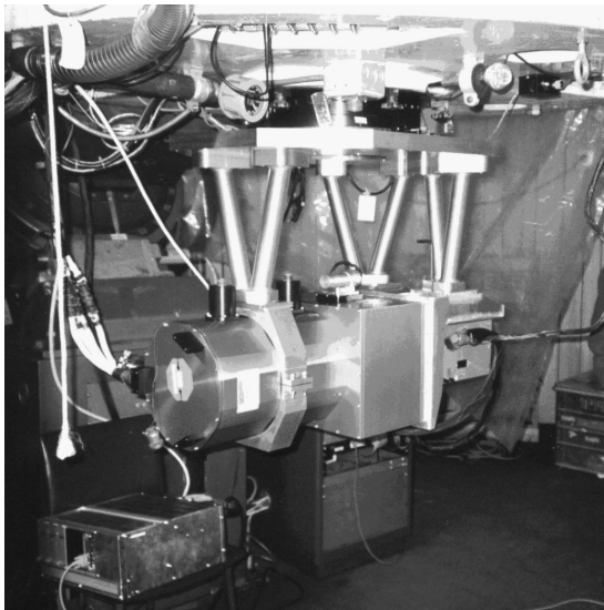
Figure 3. MIRSI mounted on the MLOF 60-inch telescope. The collar on the left hexapod has since been replaced with a direct attachment to the dewar.
