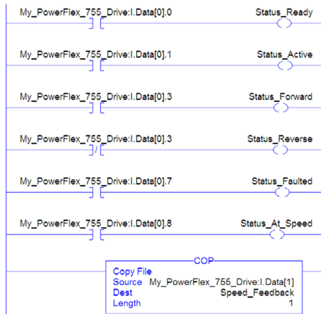
Figure 5.8 ControlLogix Example Ladder Logic Program Using Generic Drive Profiles for Logic Status/Feedback
