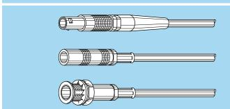
2.4 Slide the assembly into the connector shell <sup>®</sup> and screw it onto the subassembly <sup>®</sup>. Tighten using the appropriate tool to a torque of 0.25 Nm (see "Tooling" on page 31 and 32). Push the strain relief (if used) onto the crimp ferrule <sup>®</sup>.
