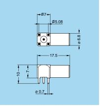
EPK Elbow socket (90°) for printed circuit with clearance under the body
