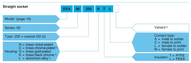
**ERA.00.250.NTL** = fixed socket, nut fixing, series 00, coaxial type (50  $\Omega$ ), outer shell in nickel-plated brass, PTFE insulator, female solder contact.
