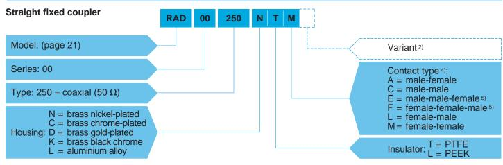
**RAD.00.250.NTM** = straight fixed coupler, nut fixing, series 00, coaxial type (50  $\Omega$ ), outer shell in nickel-plated brass, PTFE insulator, female-female contact.
