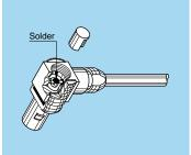
2.2 Slide the assembly into the connector shell ③ and tighten the collet nut ① using the appropriate tool to a torque of 0.25 Nm (see "Tooling" on page 31 and 32). Check that the cable conductor rests in the contact slot, solder the conductor through the hole.
