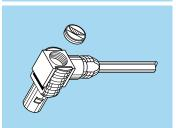
2.3 Place the insulating sleeve ④ over the soldered contact.
