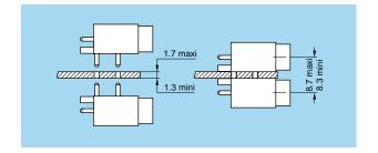
EPN Straight socket for press mounting in pair on printed circuit
