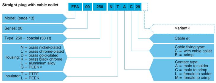
**FFA.00.250.NTAC29** = straight plug with cable collet, series 00, coaxial type (50  $\Omega$ ), outer shell in nickel-plated brass, PTFE insulator, male solder contact, C type collet of 2.9 mm diameter.
