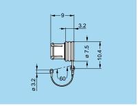
Body material: Polyoxymethylen (POM) grey Cord material: Polyamid 6, white
