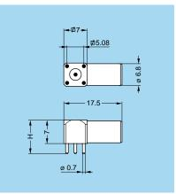
EPL-EPM Elbow socket (90°) for printed circuit
