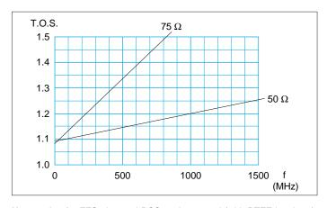
**Note:** value for FFS plug and PCS socket mated (with PTFE insulator). Impedance measured under 50  $\Omega$  with a RG-174 A/U cable or under 75  $\Omega$  with a RG-179 B/U cable.
