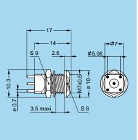
EPE Fixed socket with two nuts, for printed circuit
