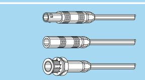
2.4 Slide the assembly into the connector outer shell ⑤. Screw the collet nut ① into the connector outer shell ⑤ using the appropriate tool and tighten to a torque of 0.25 Nm (see "Tooling" on page 31 and 32). Push the strain relief (if used) onto the collet nut.
