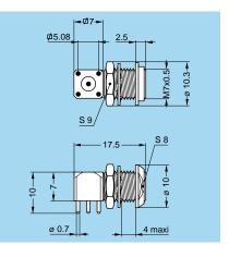
EPS Elbow socket (90°) with two nuts, for printed circuit
