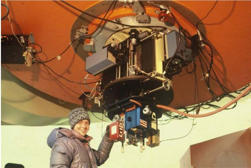
Figure 5. State-of-the-art single-detector infrared photometer (1979). Credit: C. Telesco
